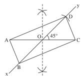
(v) With O as centre and radius -cut arcs B and D on xy.
